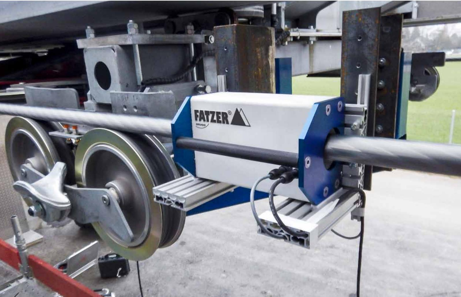
The TRUscan testing device enables wire break detection for stranded ropes up to a diameter of 64 mm.
